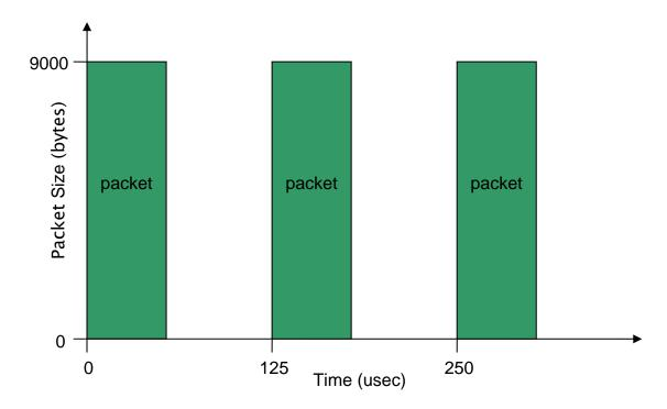
The main advantage of this approach against the Point Grey approach is that the software needs to do very little in order to be compatible – merely allow the large packets to be captured and remove the soft limit of the 8192 bytes. However, not all adapters can capture this kind of traffic reliably (it is out-of-spec after all).
